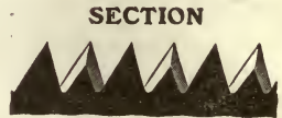
Showing actual Size and Shape of Cross-Cutting TOOTH Six Points to Inch.
