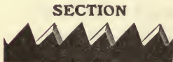
Showing actual Size and Shape of Cross-Cutting TOOTH Six Points to Inch.
