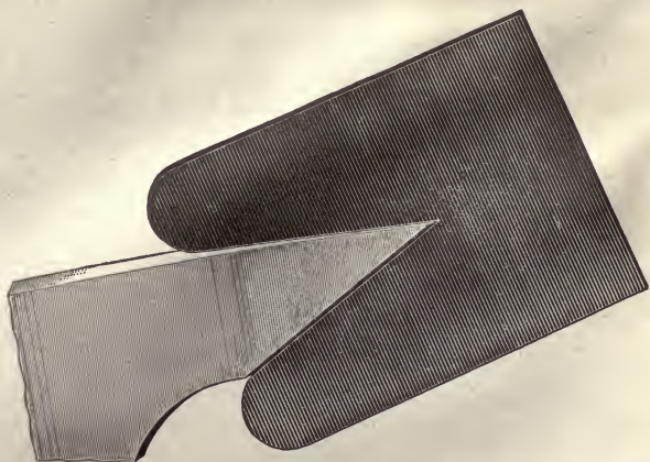
Gauge by which to File and Regulate the Shape of Saw-Teeth of Large Saws.
