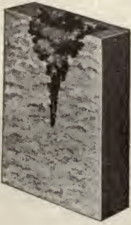
No. 1 Pipe Defect.
