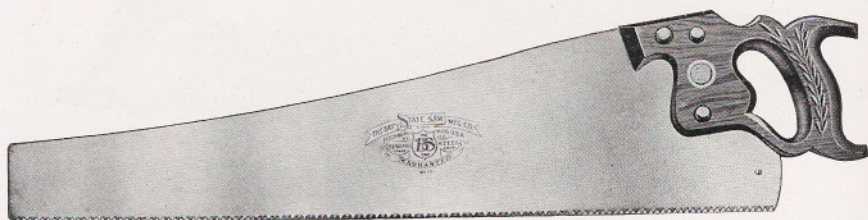
No. 25. Crucible Steel, Warranted, Carved Beech Handle, Skew Back, Four Screws.
