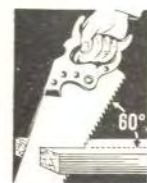
Proper angle for ripping
