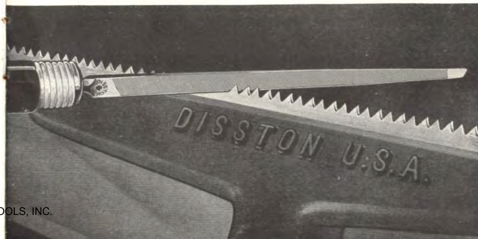
POSITION of file for beveling teeth
