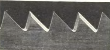
Shape of cross-cut saw teeth
