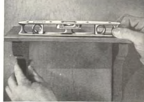
Leveling shelf with Disston A-10 Level
