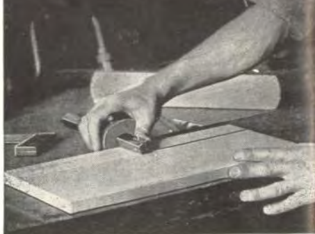
Scribing with a marking gauge
