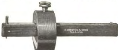
Stem showing brass plates with movable and stationary pins
