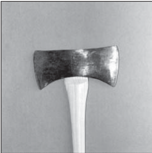
B —Saw the handle to about the correct length. The handle has been roughly fitted so the head slides to within about \frac{1}{2} inch of the final seating position.
