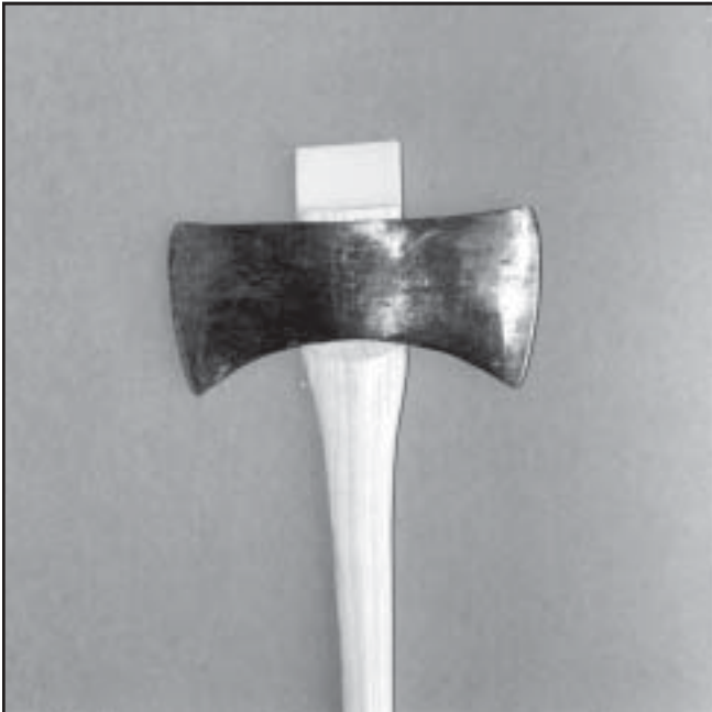
E —All surfaces just below the handle should be sanded smooth before the head is placed to insert the wedge. The wedge has been started in kerf.
