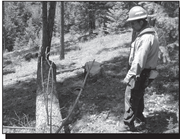
Figure 5-20—Determine the offside (usually the downhill side) and stay clear of that side when you are single bucking.
