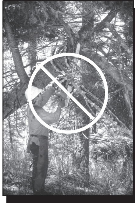
Figure 4-3— DO NOT cut with the chain saw above shoulder height. Keep the chain saw below your shoulders to maintain control when cutting.
