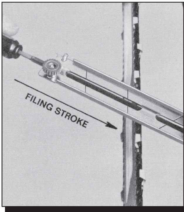
Figure 3-12—The correct top-plate angle is marked on the file guide.—Oregon Maintenance and Safety Manual, permission by Blount, Inc.
