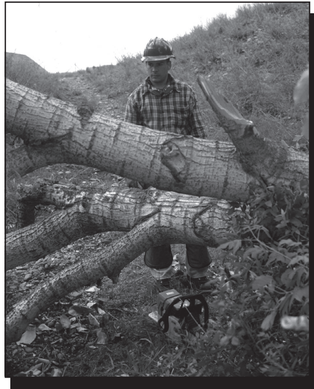
Figure 4-9—Determine the offside. It is the side the log might move to when it is cut.
