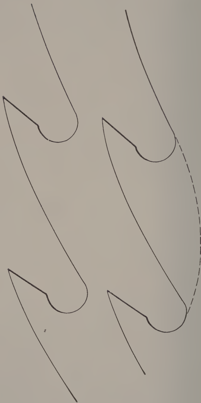
Figs. 59 and 60.—Spacing of Circular Saw Teeth.
