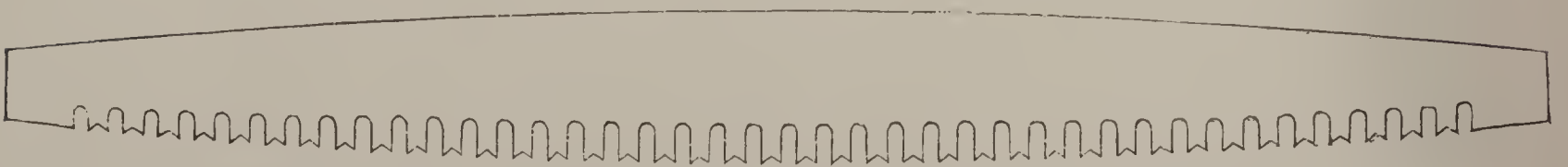
Fig. 295. Swelled Blade, with Graduated Gullets.
