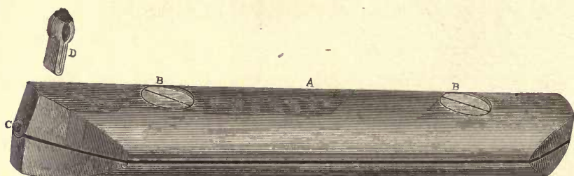
Fig. 216. Emerson's Diamond Tool for Truing Wheels.
