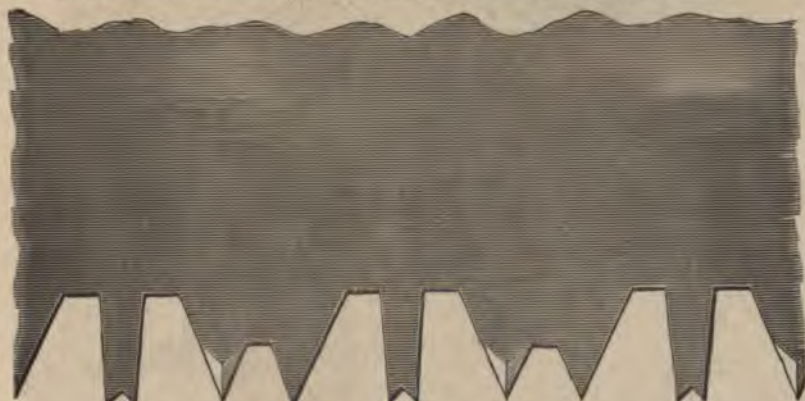
Fig. 53. "Tuttle" Cross Cut.
