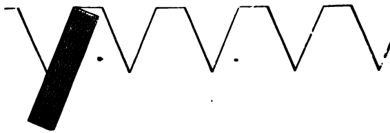
Fig. 249. Flat File on Peg Teeth.
