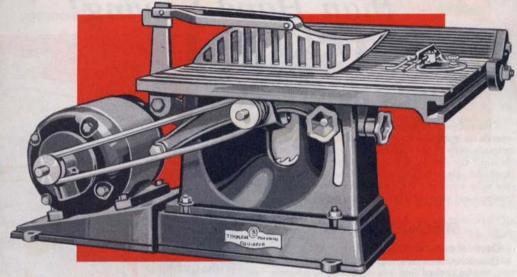
Table—17x13<sup>3</sup>/<sub>4</sub> inches, cast iron, surface ground, tilts to 45 degrees.
