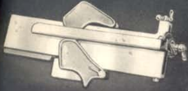
TOP VIEW SHOWING DOUBLE GUARD CON- STRUCTION USED ON THE CRAFTSMAN JOINTER-PLANNER
