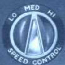
MEDIUM for non-ferrous metals: copper, brass, etc.
