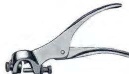
Lever saw set has a revolving anvil with indicator dial, insuring the required bevel and length of saw teeth from 4 to 16 to the inch. Hardened anvil and plunger. Finely tempered spring steel. Nickel plated finish. Weight—1 lb.
