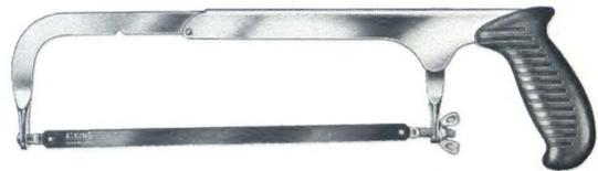
Sturdy, bright nickel frame with 3" throat. Adjusts for 10" or 12" blade in four positions. Blue handle is open pistol grip design. Blade holding bolt is equipped with large wing nut tightener and star-wheel locking nut.
