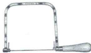
A wide throat coping saw capable of handling cuts up to 6½" in depth.
