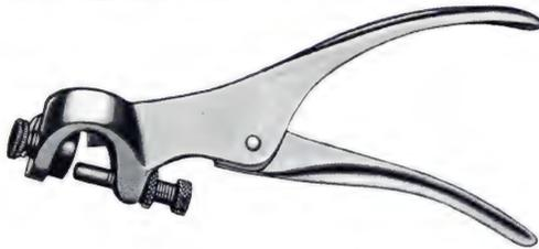
Lever saw set has a revolving anvil with indicator dial, insuring the required bevel and length of saw teeth from 4 to 16 to the inch. Hardened anvil and plunger. Finely tempered spring steel. Nickel plated finish. Weight—1 lb.
