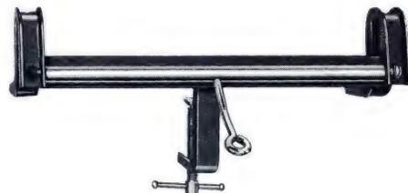
Clamps on any board or bench. Sturdy for long service. Saw is held between strong steel channel section and eccentric rod. Grease and oil resistant, chatter-free fibre insert is riveted in four places to channel section, giving double grip on saw. Filing space is  $10\frac{1}{2}$ " long. Weight,  $2\frac{1}{4}$  lb.
