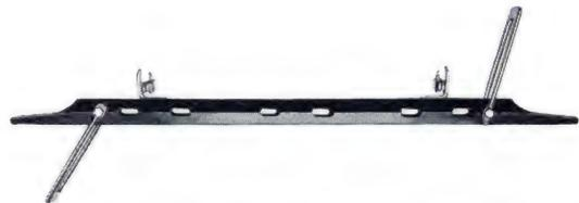
Grips the entire length of saw—30 inches. All steel. Gripping edges are ground and hold saw true—no vibration. Also holds band saws. Can be attached and removed from bench in 15 seconds. Weight,  $4\frac{1}{2}$  lb.
