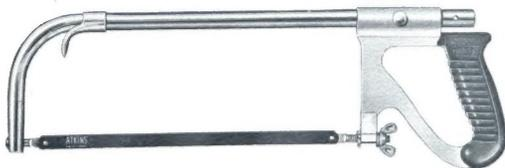
Fine looking, well balanced frame of tubular steel, featuring the popular knuckle-guard design and blue acetate handle. Frame is polished chrome on nickel with 4" throat, adjustable for 10" and 12" blades. Blade bolts have safety clip and star-wheel locking nut. Adjustable thumb rest for 2-hand use. Individually packed and equipped with ATKINS blue lacquered steel blade. Weight, 1¾ lbs.
