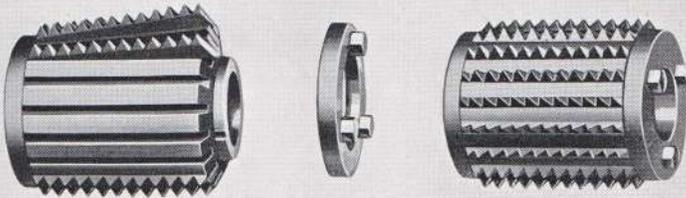
Enlarged Sections of Lath Mill Roller
