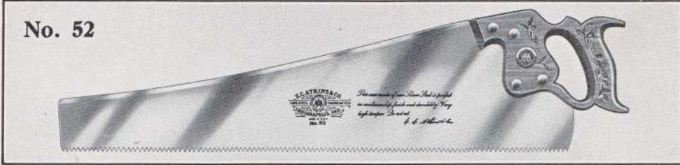
This saw is made for fine cabinet work, where a very smooth cut is essential. It is given an extra fine hard temper, so that the teeth may be sharpened to an extremely keen cutting edge. It is ground five gauges with an extra thin taper back, also slightly hollow, which gives it ample clearance. The teeth are sharpened to a needle point. *It runs without set.* Blade skew back, Atkins Silver Steel, high polish.
