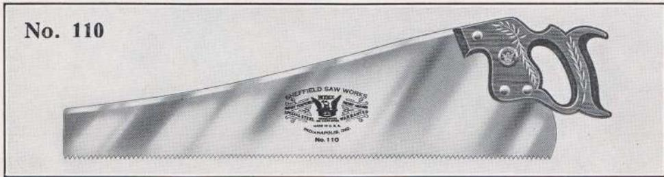
The No. 110 is a popular price Hand Saw made to meet the demand for a medium price, good quality saw. It is made from Crucible Steel, full width, high polish, skew back, ribbon edge, cherry handle; spindle carved, attached with four brass screws and medallion.
