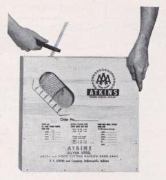
This is the sturdy, familiar, wooden case used to pack Wood, Butcher, and Metal Cutting narrow band saws in standard 250 feet coils. Any length of the coil may quickly be removed. The number of feet remaining in the case is always shown on the front as well as the specification of the contents.
