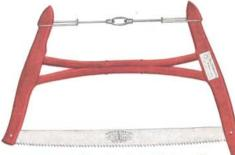
No. 40. Disston Wood Saw, Stained Red and Varnished, 30 inches. No. 26 Round-Breast Blade. Thin Back, 23 inches wide, 41 Points. Climax Rod, Plain.
