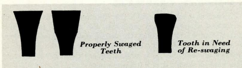
top clearance, will run hard and pound in the cut. Before swaging, points should be brought up to a sharp edge.
