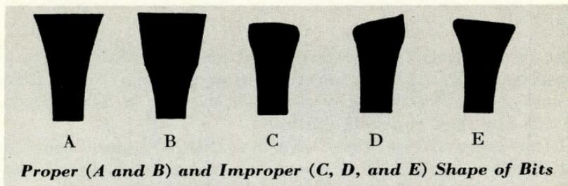
**Filing the teeth.** Never file so as to lower the point of the tooth, for this will cause the saw to buckle and refuse the feed. After a set of teeth has once been jointed, NEVER file on the top to sharpen except when necessary after jointing. The short bevel caused by jointing should be removed by filing but be sure to hold the file flat on the entire top of the tooth so that you remove as much metal from the heel as at the point. The original top clearance must be maintained.
