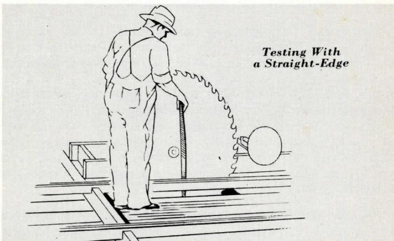
**Test with straight-edge.** Try the log side of the saw with a long straight-edge to see that it is flat.
