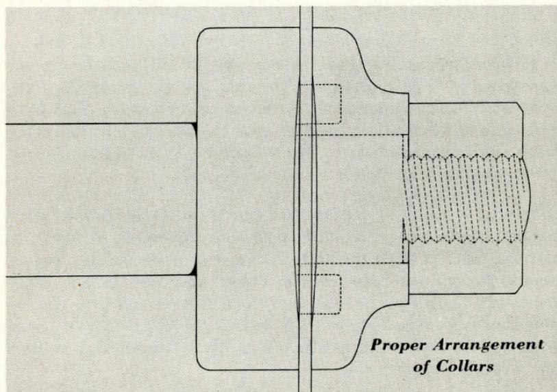
**Shape of the fast collar.** The fast collar should be perfectly true, but slightly concave on the face; just enough to show light under a straight edge. This is to insure that the outside rim of the collars will grip the saw.
