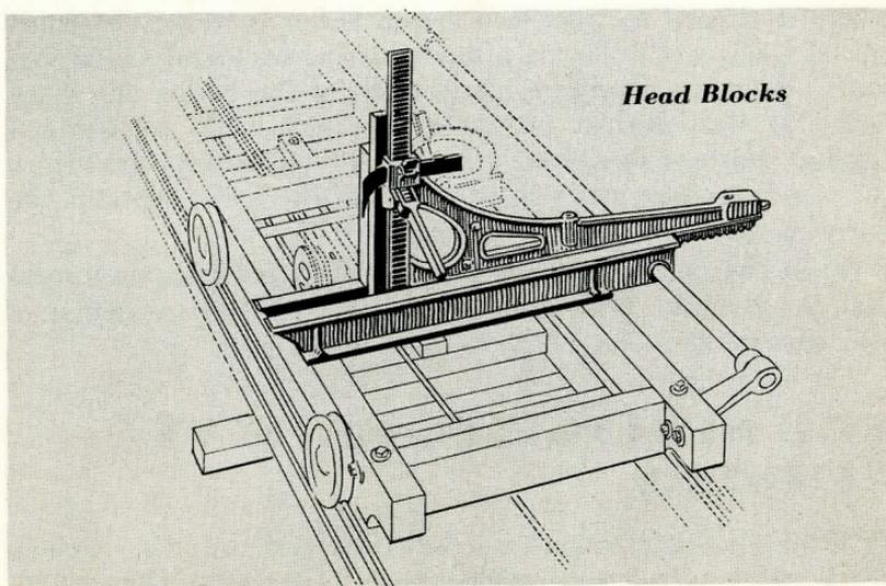
**Testing head blocks.** Run the carriage its entire length with a level on each head block to see that carriage will pass the saw without rocking.
