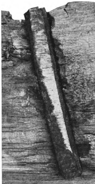
Spike Sliced by Disston Heading Saw.
