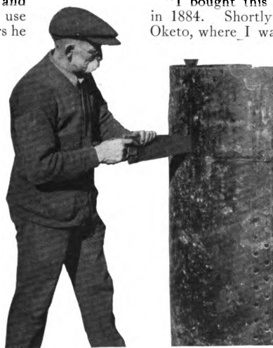
A Disston 22-Inch, 8-Point Hand Saw, made for cutting wood, used for cutting boiler plate
