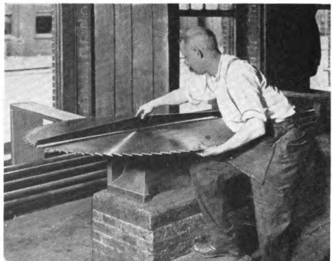
Figure 9—Appearance of a saw that has lost its tension. Notice the space between straight edge and rim of saw.
