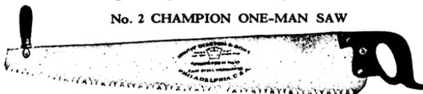
A very good medium priced saw, popular with those who do not have constant use for a one-man saw and with whom ordinary speed in cutting meets the demand. Medium-width blade. "Two-cutter" type and has large grip handle. Made of Disston-made steel. Ground two gauges thinner on the back than on the tooth edge. Regular lengths 2½ to 6 feet, or longer if desired.
