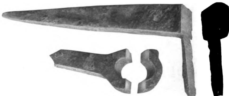
**T**HE gate hinge shown above was embedded in a walnut log which was being cut in the Hoosier Veneer Co., of Indianapolis, Ind. It was struck by a DISSTON band saw with the result above illustrated. It is of course not an uncommon thing to strike metal in making a cut but the peculiar part of this cut is its absolute symmetry. It could hardly have been cut more squarely along the center if it had been measured.
