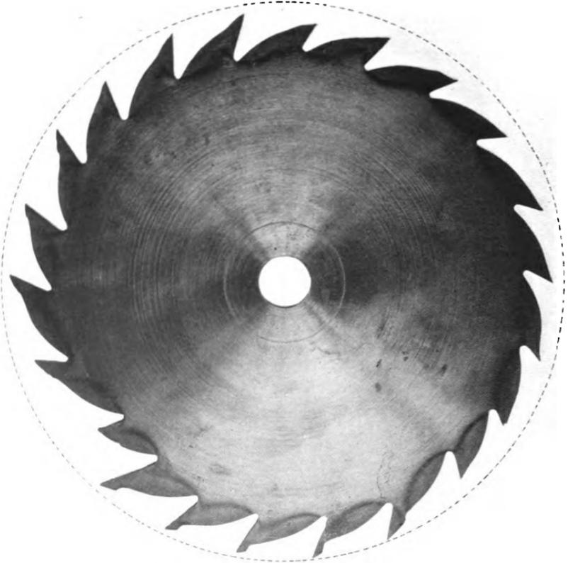
**T**HE saw shown above is presented as a fine example of masterly handling. Close scrutiny reveals with what infinite pains all semblance to the original shape of the teeth has been obliterated, and no two teeth in this saw have been left the same length, as so frequently happens in ordinary saws. The elliptical shape doubtless was imparted to make the saw run as unevenly as possible in the cut, thus obviating the monotonous
