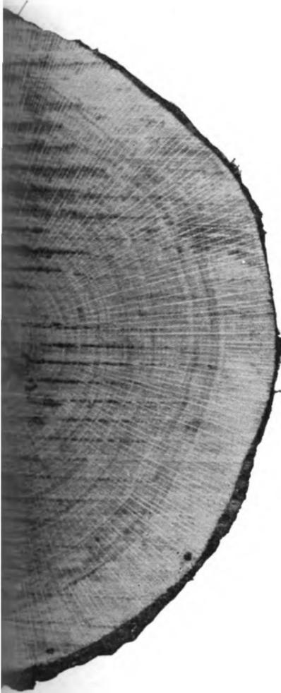
white oak, and the cutting, approximating 1 inch a second, demonstrates the advisability of the use of a high-grade saw of this character, when the operator desires to save time and labor.
