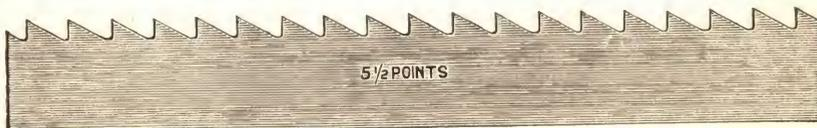
The following cuts are full size of the respective number of teeth and points per inch which they represent. It will be noticed that in one inch space, there is one **tooth** less than there are **points**. Order all saws by the number of "POINTS" to the inch, measuring from point to point of teeth.
