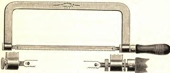
Solid steel back 1 inch x  $\frac{1}{4}$  inch, depth  $5\frac{1}{4}$  inches from inside edge of frame to tooth edge of blade, Polished Hardwood Handle. This is the strongest frame made. No riveted parts. Reversible stretcher, special adjustment, sockets of solid steel forged. Made for 12 inch blades only.
