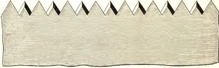
no pitch at all ; the angle on each side being the same, forms the "*peg tooth*," which is best adapted to cutting soft, wet and fibrous woods. This style of tooth is principally used in Buck-saws.
