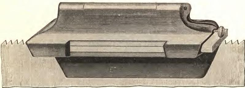
When the teeth of a saw become irregular in size it is absolutely necessary to dress them down until all are of an equal height, and this should always be done before attempting to reset or sharpen the saw.
