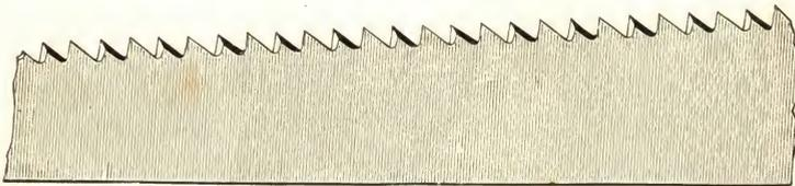
Fig. 18 is a section of a pruning saw which differs from a cross-cut hand saw in being thicker, having a little more pitch to the teeth and
