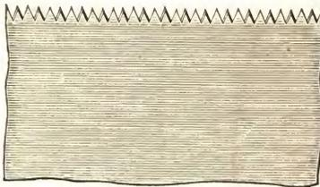
Fig. 17 is the finest toothed saw of its kind that is made for wood. All the above mentioned saws in Figs. 14, 15, 16, and 17, are made especially hard and will not admit of setting, but being made thinner at the back, when properly filed, will cut clean and sweet. Teeth such as shown in Fig. 17 are used principally on Back Saws and smooth cutting hand saws. To maintain the original shape of these teeth use our cant safe back file.
