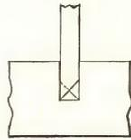
Fig. 4 shows how the groove should appear on looking down the edge of the saw; the action should be such that the bottom of kerf will present the appearance as shown in Fig. 5, and not like Fig. 6; the cutting action is as shown in Fig. 7, the cutting being done with the outside of tooth, the fibre of the wood is severed in the two places and the wood is crumbled out from point to point by the thrust of the saw.
