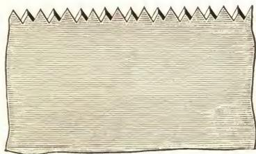
Fig. 14 is a section of an eleven-point saw suitable for the finer kinds of work on dry, soft woods, such as cutting mitres, dove-tailing, pattern work, etc.
