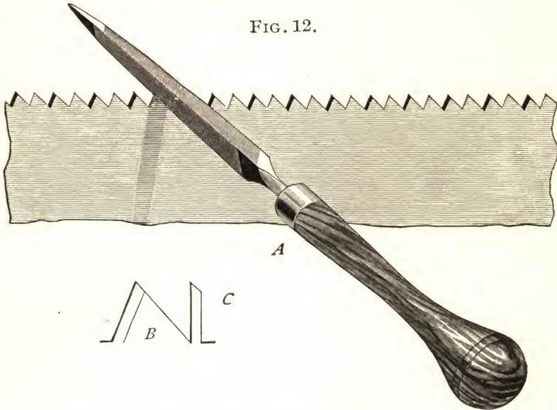
Fig. 12 is a still finer saw, having ten points to the inch. This saw has no fleam on back, the result being very noticeable at *C* and *B*. This style of point is for hard wood.
