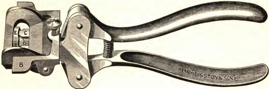
The idea embodied in this Saw-Set is one that will commend itself to every user of a saw-setting tool. The principal feature is the use of two plungers operated by the two levers or handles; pressure on the lower lever forcing plunger "D" against the body of the saw, thus holding it rigidly in position and preventing slipping, whilst a continuation of the pressure on the upper lever operates plunger "C" in setting the tooth.
