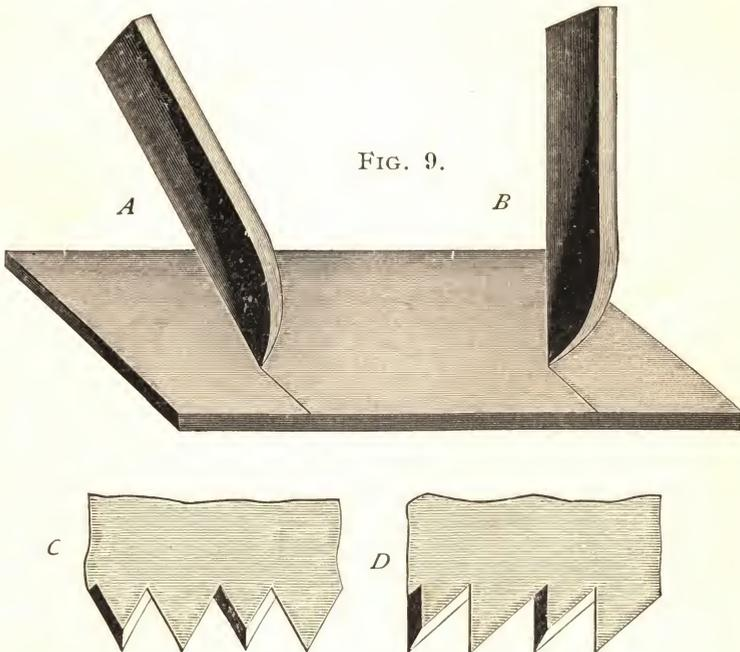
we hold the knife nearly perpendicular as at *B*, it is evident it will push harder and will not cut as smoothly as if it was inclined forward as at *A*; it follows then that the cutting edge of a cross-cut saw should incline forward as at *C*, rather than stand perpendicular as at *D*.
