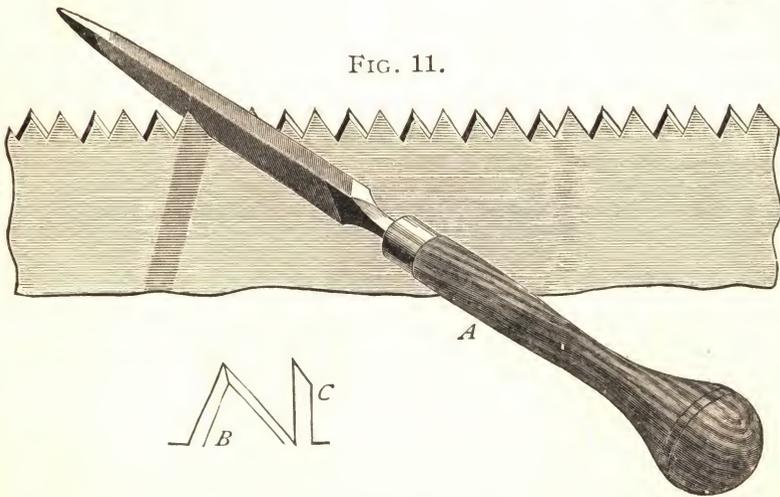
horizontal to the perpendicular of the side of saw, and on an angle of about  $45^\circ$  longitudinally with the length, measuring from file line toward heel.
