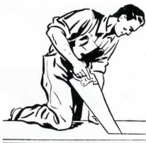
Proper position for ripping
