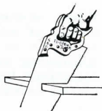
End of downward stroke should be 6" to 8" from butt of blade
