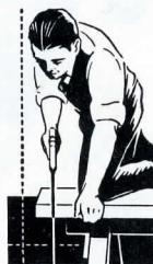
Proper position for cross-cutting
