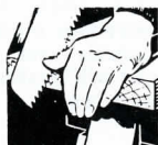
Start cut with a draw stroke, and use thumb to steady blade
