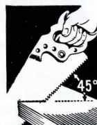
Proper angle for cross-cutting
