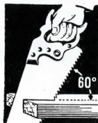
Proper angle for ripping
