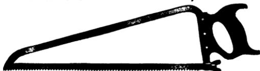
Flat steel back, narrow tapered point, Beech handle, three brass screws. Handle has extra large hand-hold for use in gloved hand. Blued steel blade, 18½ inches long.
