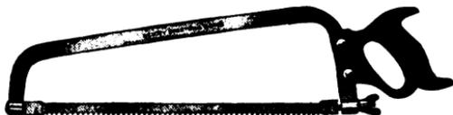
Flat steel frame, slightly tapered, riveted sockets, swivel stretcher. Beech handle, two nickel-plated screws. Blued steel blade. Length 14 inches centre to centre of holes.
