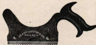
This special saw is for trenching out stringers, making slots in stair treads or risers, and similar work. The blade is of Disston-made Steel and is adjustable in the back so that an even, accurate cut of specified depth can be made. The blade is removable so that the owner may use the same handle with new blades.
