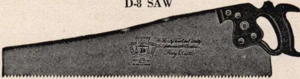
This is the best and most popular Disston Saw for general, all-around work. It is "the saw most carpenters use." The D-8 is the original skew-back saw originated and patented by Henry Disston in 1874. The shape of the blade and the position of the handle place the hand closer to the work, and, therefore, give the user better command and guidance of the saw, allow him to make a full stroke, and give more power to his cutting strokes.
