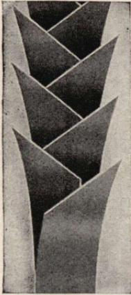
Tooth edge of saw for cross-cutting
