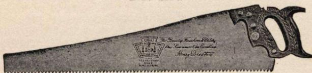
The D-20 saw is made particularly for those who prefer a narrow width blade. This blade, skew-back in design, is  $1\frac{3}{4}$  inches wide at the point and  $6\frac{1}{4}$  inches at the butt instead of  $2\frac{3}{4}$  inches at the point and  $6\frac{3}{4}$  inches at the butt as in the D-8. This makes the D-20 a very light and easy saw to operate. This feature, together with the comfortable grip, makes the D-20 a favorite with some users.
