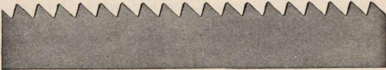
Section of 6 point saw for cross-cutting
