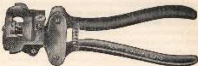
Fig. 19.—Triumph saw set for circular saws.
