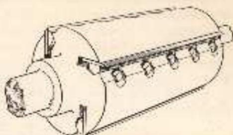
Fig. 104.—Round cylinder head with four thin high-speed knives.
