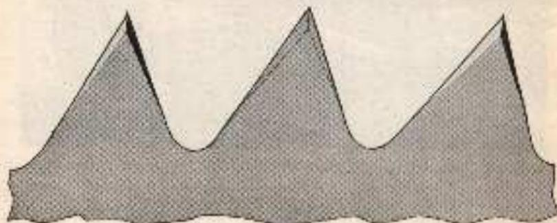
Fig. 41.—Bevel and angle of teeth of circular cross-cut saw for hardwood, magnified.
