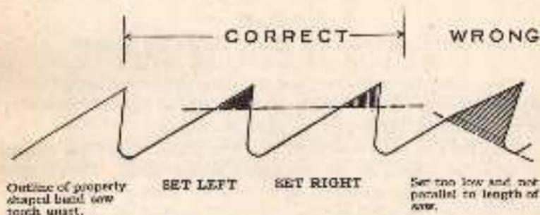
Fig. 35.—Proper setting of narrow band saw teeth.
