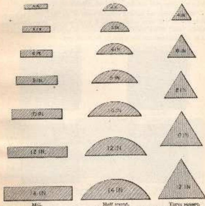
Fig. 81. Actual cross-sections of files for lengths indicated.
