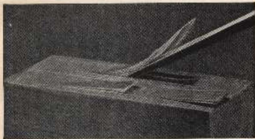
Fig. 12.—Comparing action of rip saw tooth with a chisel.
