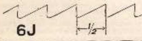
Fig. 31. — Proper shape for narrow band saw teeth, showing  $\frac{1}{2}$ -inch space.
