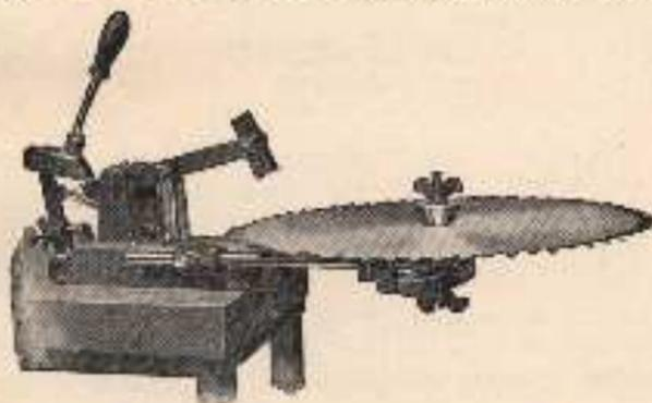
Fig. 188.—Setting machine for circular saws.
