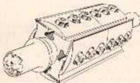
Fig. 103.—Thin high-speed knives and ends with notched square head.
