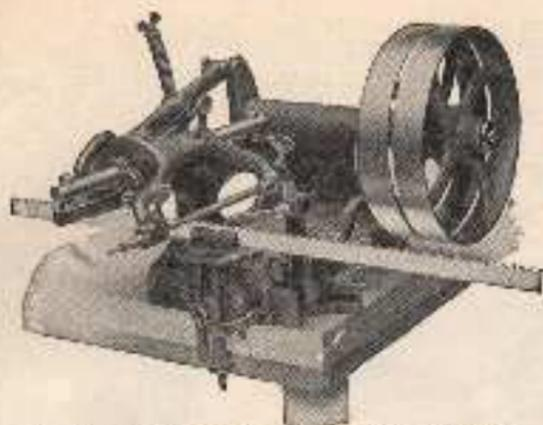
Fig. 178. Band Saw Trimmer Machine (power driven).
