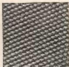
Fig. 79.—Rough cut of double-cut file.
