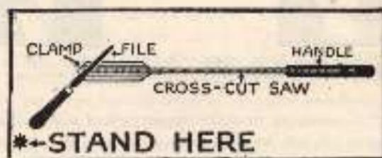
Fig. 25.—First position for filing cross-cut saw.
