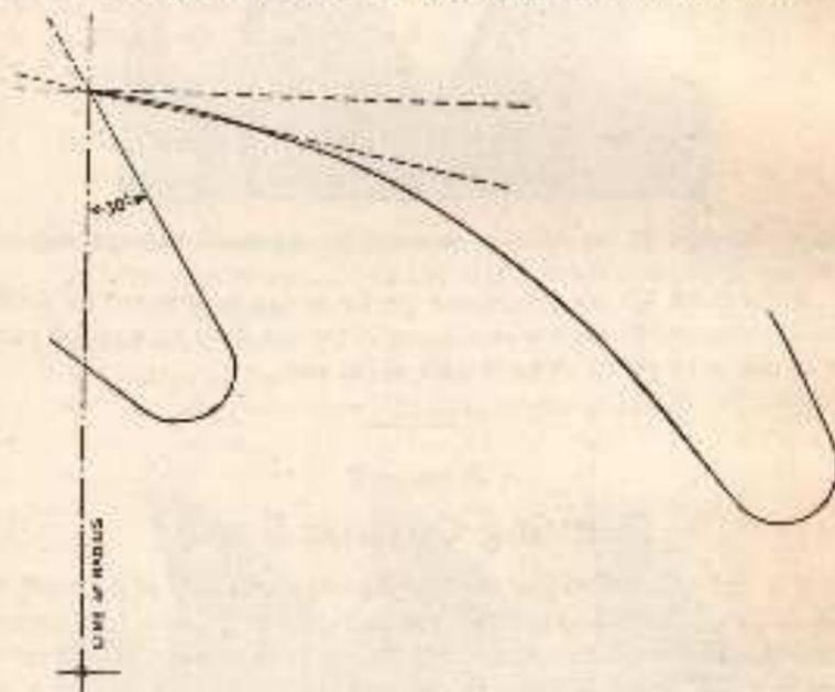
Fig. 44.—Correctly designed rip saw tooth.
