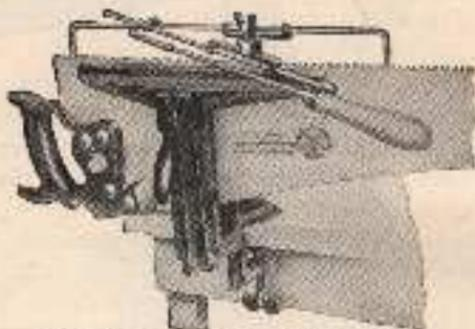
Fig. 194.—D-3 Saw Filing Guide and Clamp.
