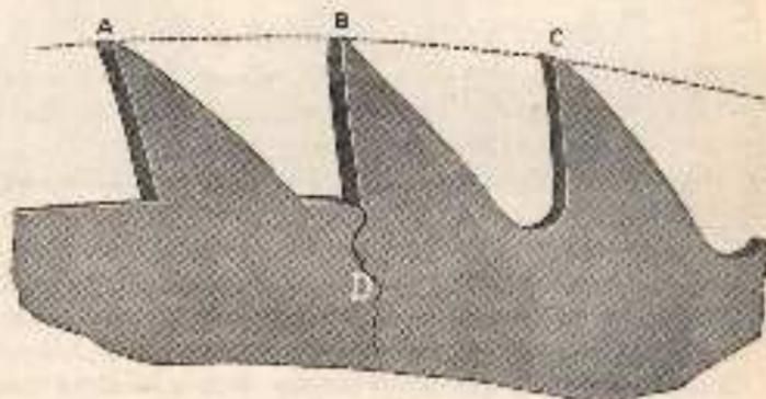
Fig. 42.—Crack resulting from square gullet, magnified.
