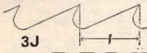
Fig. 32. — Band saw teeth showing back (1 inch space).
