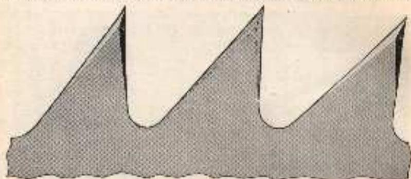
Fig. 40.—Bevel and angle of teeth of circular cross-cut saw for softwood, magnified.
