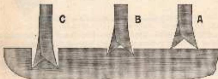
Fig. 10.—Scoring and cutting of cross-cut teeth (end view).
