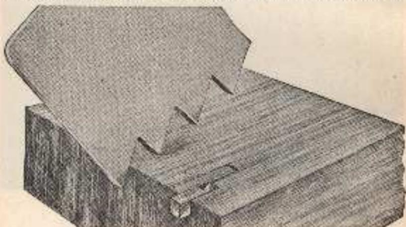
Fig. 13.—Action of rip saw teeth.
