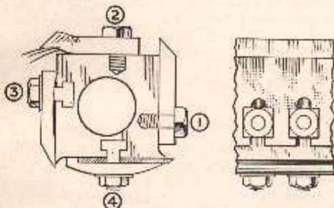
Fig. 102.—1, First method of attaching square head knife; 2, buckling due to flat face; 3, properly attached knife with concave bearing surface; 4, adapting head to thin high-speed knife.
