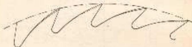
Fig. 47.—Bevel on back of circular rip teeth.
