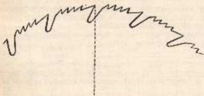
Fig. 37.—Standard section of new circular combination saw.
