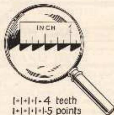
Fig. 27.—Method of determining points per inch.
