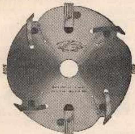
No. 143.—A new and better Saw, combining in one tool a Groover, a Dado Head, and a Shaper.
