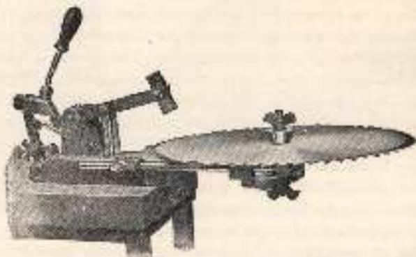
Fig. 22.—Machine for setting circular saws.
