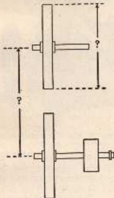
Fig. 176. Necessary measurements for figuring length of band saw.
