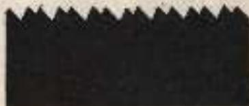
Fig. 21.—This saw needs jointing.
