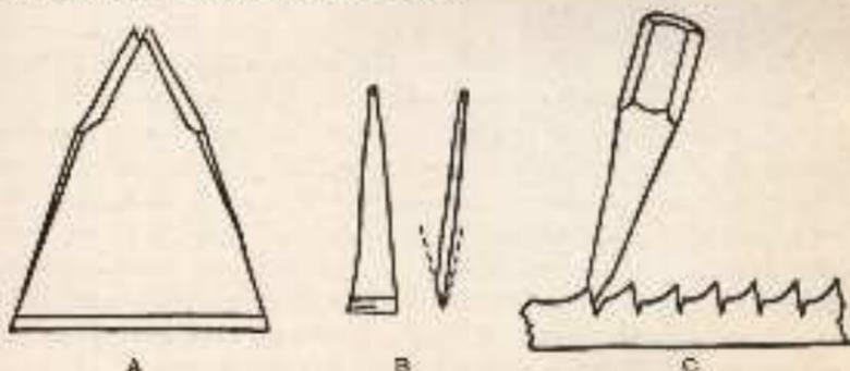
Fig. 94.—A, Chisel for handcutting large, rough files; B, chisel for cutting small, fine files; C, action of chisel in upsetting teeth.
