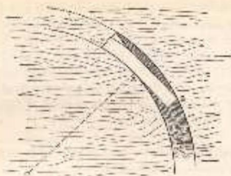
Fig. 30.—Section of hand saw in curved cut.
