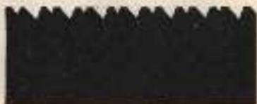
Fig. 22.—The saw in Fig. 21 after jointing. Shape the teeth next.
