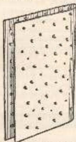
Fig. 89.—Indian rasp used in making arrow shafts.
