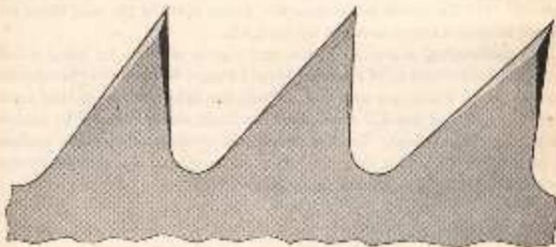
Fig. 48.—Correct "fitting" of circular cross-cut teeth.
