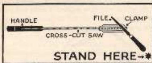
Fig. 26.—Second position for filing cross-cut saw.
