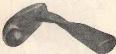
Fig. 94.—Hammer used to cut files by hand.
