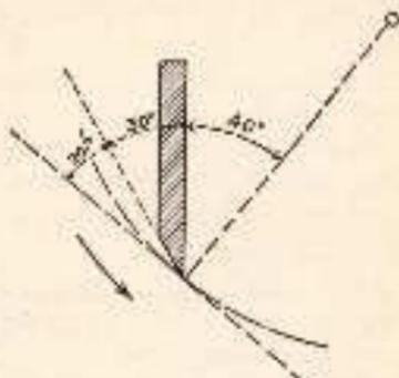
Fig. 100.—Cutting angle of high-speed steel machine knife.
