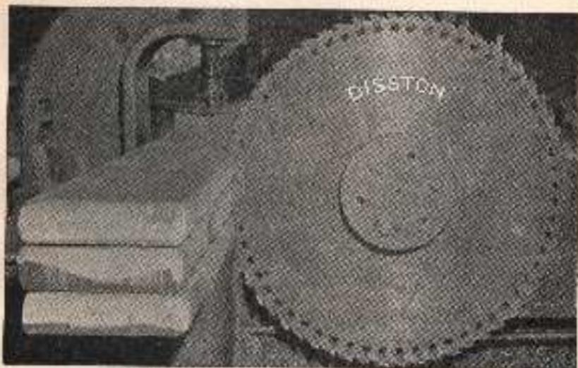
Fig. 72.—Fifty-inch inserted tooth metal cutting saw.
