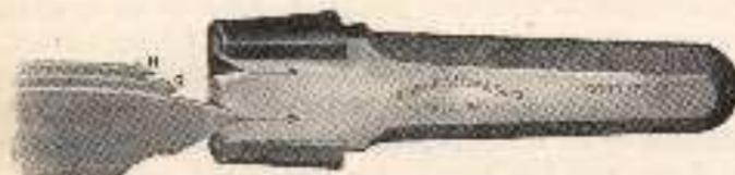
Fig. 53.—Conqueror swage for circular saws.
