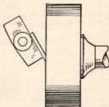
Fig. 107.—Grinding flat bevel on machine knife.
