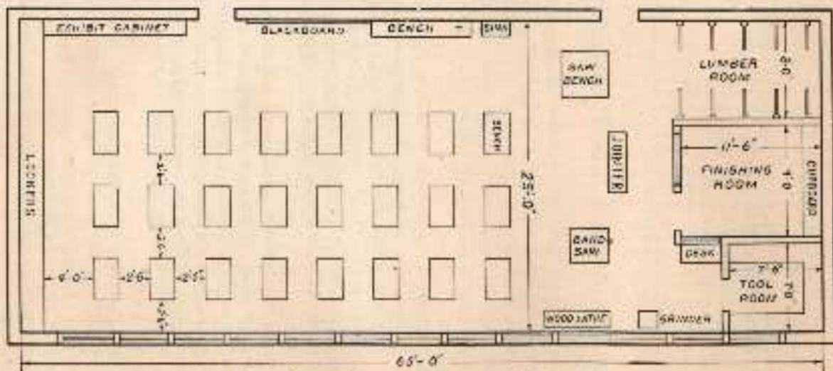
Fig. 1.—Suggested layout for 24-bench woodworking shop.
