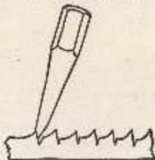
Fig. 78.—Showing angle of chisel in cutting file tooth.
