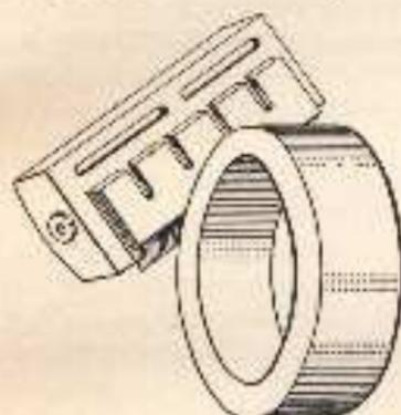
Fig. 106.—Grinding concave bevel on machine knife.
