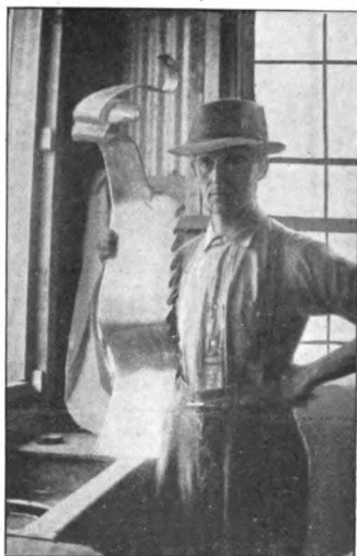
This picture shows the curious and peculiar manner in which a Disston Bandsaw broke in Bathurst Lumber Co.'s Mill No. 2. All twisted up, and the filer says he never saw the beat of it for toughness
