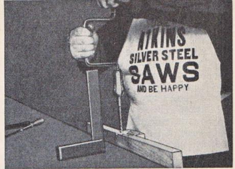
Fig. 27—Boring holes for a staggered dowel joint
