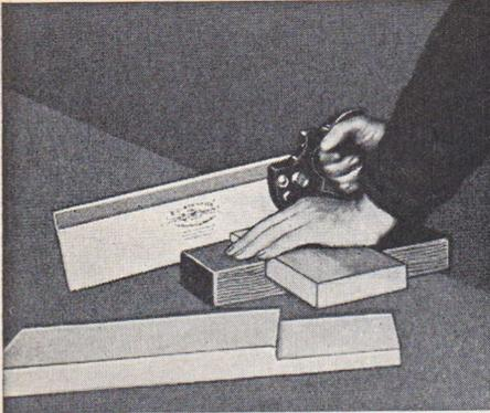
Fig. 13—Cutting shoulders of half lap joint with ATKINS Silver Steel Back Saw No. 2, in bench book
