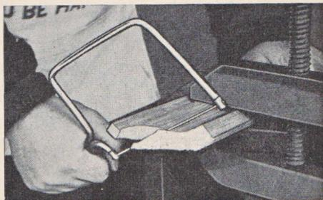
Fig. 35—Using the ATKINS Silver Steel Coping Saw No. 100 to cut moulding for a coped joint
