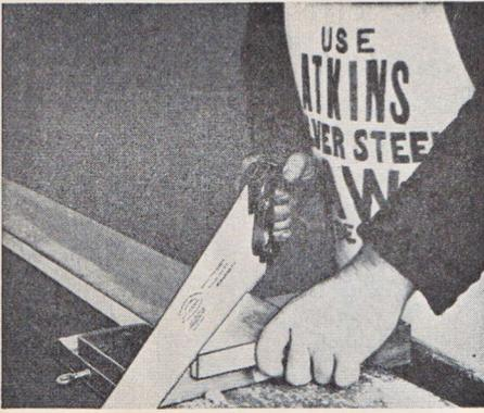
Fig. 18—Cutting a miter joint with ATKINS Silver Steel Panel Saw No. 53
