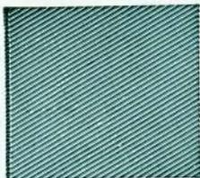
A Single-cut File has single rows of parallel teeth extending the length of the file at an angle across its face. This is clearly shown in the illustration.
