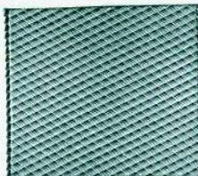
other. The first row is usually coarser and deeper than the second row. The first row of teeth is known as the "over cut" the second is the "up cut." The teeth of a double-cut file are sharp points as shown here. For this reason they cut faster but not so smoothly as the single-cut. Most of the files used by machinists are double-cut.
