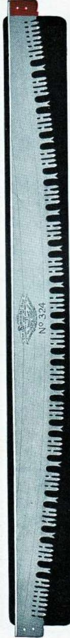
No. 324. Lance Tooth. Four Cutting Teeth to each Raker.
