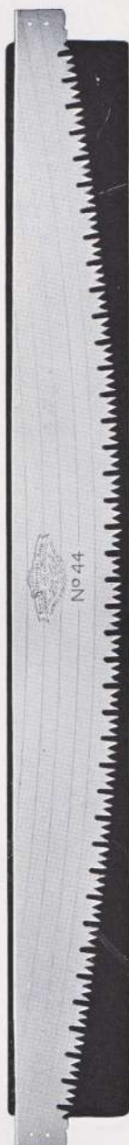
No. 44. Roomy gullet between each set of 3 teeth that readily carries the sawdust from the cut.
