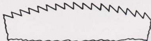
"V" TOOTH on small saws with less than 1/8" space
