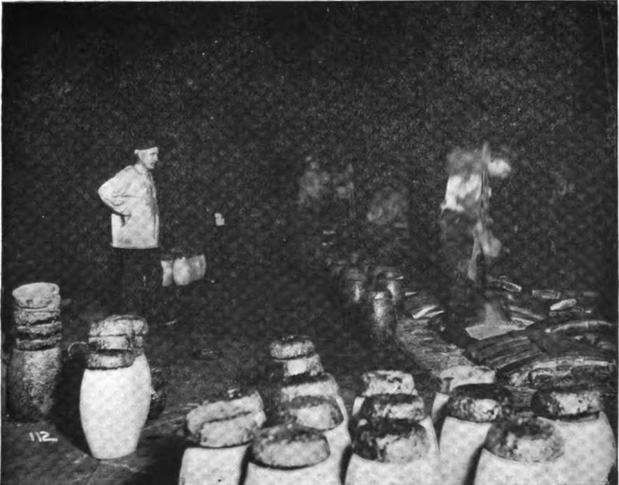
Hot work. Placing full crucibles in furnaces
