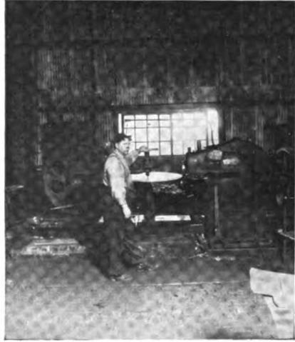
Circular Shear rounding plates for the saw factory
