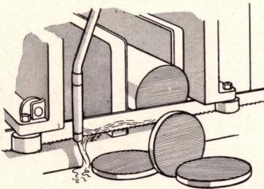
This carbon alloy type steel blade has been specially heat treated so that it has a spring temper back with a full hard cutting edge. As a result, it has nearly twice the tensile strength of ordinary carbon steel blades. This means you can place it under greater tension
