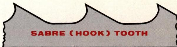
This design is similar to, but offers two distinct advantages over, the Skip Tooth Saw: (1) the face or cutting edge of the tooth has a 10° hook which makes the saw feed easier; (2) its chip breaker design prevents soft, gummy materials from sticking in the gullet. Used on essentially the same applications as Skip Tooth, the Sabre Tooth Saw will do more work at lower cost.
