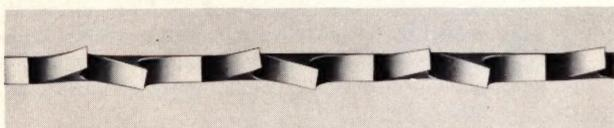
Regular Set is generally furnished on saws which have 2 to 24 teeth per inch. Saws with Regular Set have one tooth set to the left, one to the right and one tooth unset, called a raker. This type of set is used where the material to be cut is of uniform size and for contour cutting.
