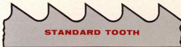
Standard Tooth Saws, with their well-rounded gullets (see illustration above), are best suited for cutting most all ferrous materials as well as nonferrous materials such as hard brasses and bronzes. This style tooth is also used for friction sawing.
