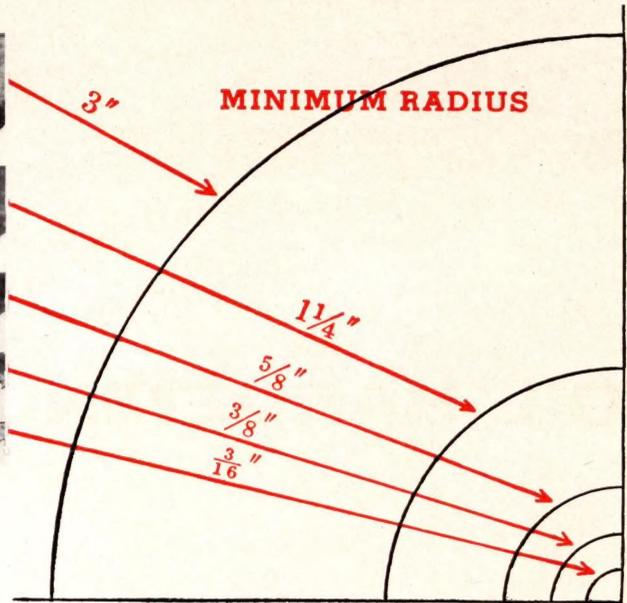
In contour sawing the radius of the curve to be cut governs the width of the saw to be used. The smaller the radius, the narrower the blade. For desired radius use width of saw as indicated by above chart.
