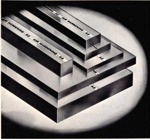
Simonds offers an Air Hardening type of Die Steel for longer lasting punches and dies where greater production runs are desired between sharpenings. This 5% chrome type steel will produce up to 50% more pieces per sharpening than the Oil Hardening type of Die Steel. Due to the Air Hardening features less skill is required in heat-treating.
