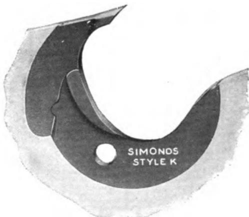
The special feature of this tooth is that a greater number of teeth may be carried, yet each tooth has a large open gullet. An examination of the construction of the tooth will show this large gullet room and also a swaged shank to aid in carrying off the sawdust and keeping the plate cleared. Points, shanks, and plate have a close fitting machine milled "V" and groove.
