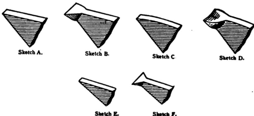
Where there is such a large amount of material in the tooth, it requires double the amount of pressure to spread it. In fact, it does not spread clear through the tooth, but simply rolls the metal over at each side of the tooth, extending quite a distance down the back of the tooth, with scarcely any in front.
