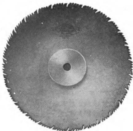
**Novelty Saw.** The novelty saw can be made for either rip or cut-off work. When used for ripping the teeth should be so that when a straight edge is laid across the center of the saw it will also be in line with the front of the teeth. For cross-cutting exclusively a "V" tooth is better.
