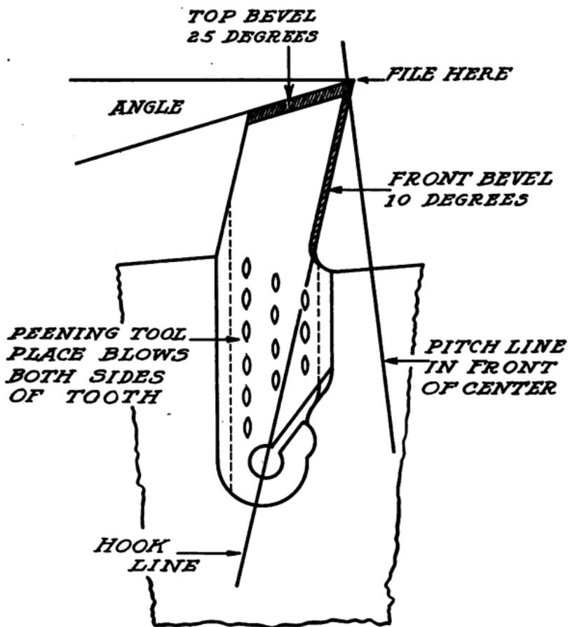
case with some slasher, trimmer, and circular gang saw rigs. The hook can be taken out and any degree of pitch in front of the center given by simply filing the point of the tooth to the desired angle. It is not necessary to file a long pitch line— $\frac{1}{16}$  to  $\frac{1}{8}$  inch is enough. This does not reduce the cutting wear of the tooth.
