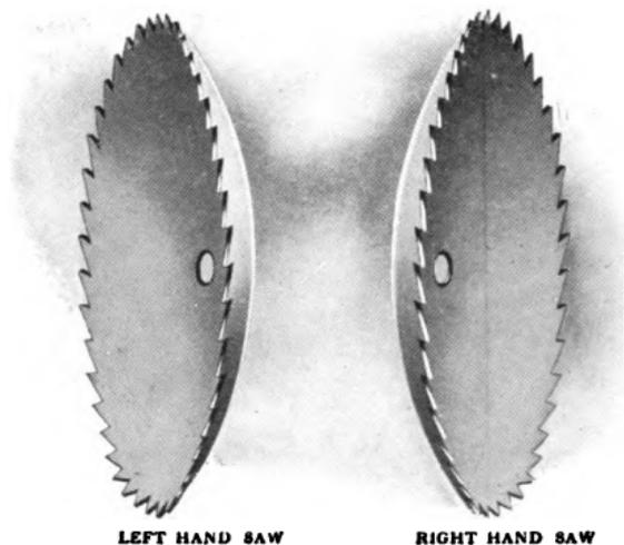
When ordering Concave Saws give circle to be dished to, or give the diameter of the old saw and the amount of drop in the old saw, accurately measured; also give the greatest diameter of the heading to be cut. State which side is to be dished or concaved, right or left hand, as the saw runs towards you
