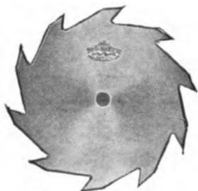
**Grooving Saws.** These saws are ground thinner at the center than at the rim, so that little or no set is required or just enough to keep the extreme points of the teeth perceptibly wider than the body of the teeth. We make them any gauge at edge or center, as ordered.
