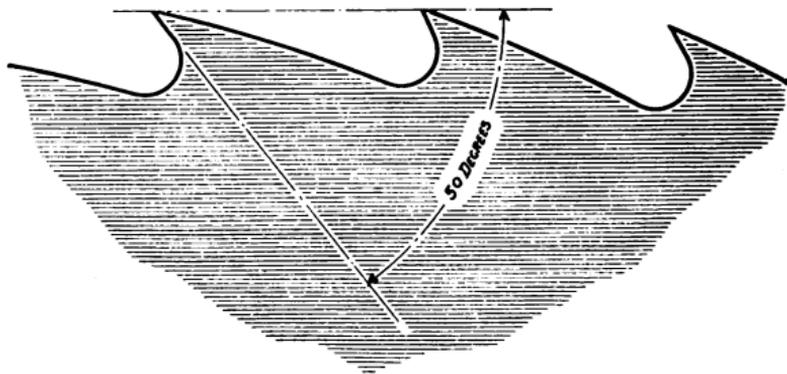
This sketch opposite is a good one to use as a guide for the proper shape of shingle saw teeth. Notice that one line is drawn straight across two teeth and one drawn following the hook of the tooth. The angle formed is 50 degrees.
