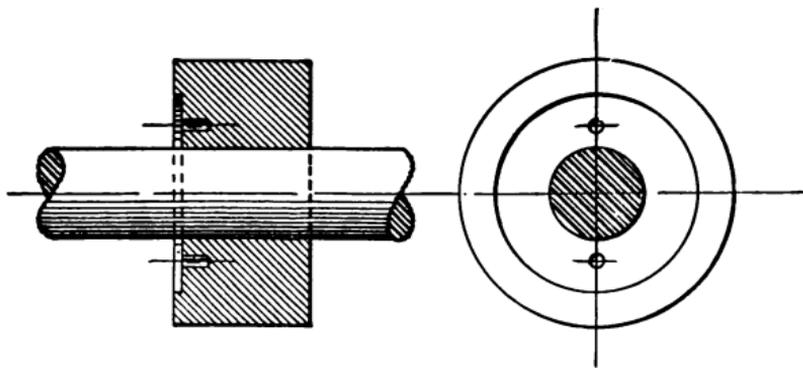
The saw should slip freely on the mandrel and close up to the fast collar. In many cases where the stem of the
