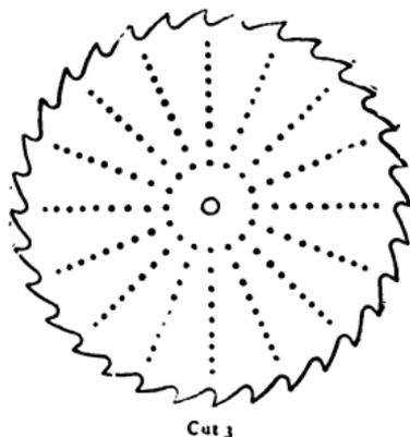
If, however, in the process of regulating the tension, you find the saw to be a trifle dishing, lay it on the anvil with the full side up, and hammer lightly over body of saw, as in Fig. 3 until you have made it perfectly flat on the log side.
