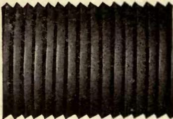
Fig. 53.—"Cut" used for filing handles.
