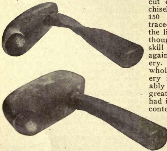
Fig. 22.—These are typical hammers used by hand-file cutters. The grooves in the handle of the smaller hammer have been worn in by the grasp of the hand through many years' use.
