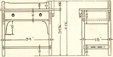
plane the bottom shelf 36" long, 13" wide, 1" thick; cut tenons to fit mortises. Cut two pieces for the back each 36" long, the first piece 8" wide, the second 5" wide, the tenons of which are 1" long. Mark out design on the top piece and cut out with a turning saw; smooth with a plane and wood file; scrape and sandpaper until all parts are smooth. Glue and clamp together; clean off glue.
