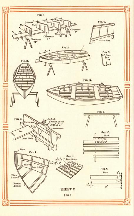
Next come the blocks for oarlocks, shown in Fig. 8 (Sheet 2). Along the whole length of boat at top of the side boards and stern is a strip called the fenderwale. It is shown in the drawing marked "stern view" on Sheet 1. The keel is also shown. It is a hard board, nailed to the bottom of the boat.
