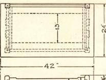
Cut side pieces 20" long. The lower one is 3" wide and the upper one is 10" wide; the tenons are 1" long; find the middle of these bottom pieces, measure 1" on each side of the middle and lay out and cut mortises for the bottom shelf 3" long, 3%" wide.
