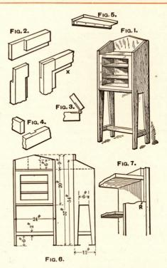
If yellow pine is used, to finish the cabinet in natural style apply three coats of varnish, the first and second thinned out and the last full strength. If it is desired stained, put on two coats of stain after the first filler coat of varnish, and after the stain either wax it or varnish it. For open grain wood like oak, use paste filler first, thinning stain and varnish.
