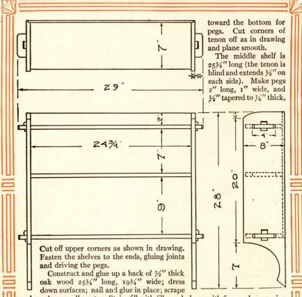
and sandpaper all parts. Stain, fill with filler, rub down with fine sandpaper, give a thin coat of shellac and wax.
