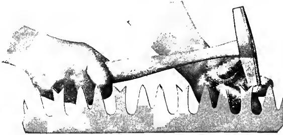
FIG. 2. METHOD OF SWAGING RAKERS
