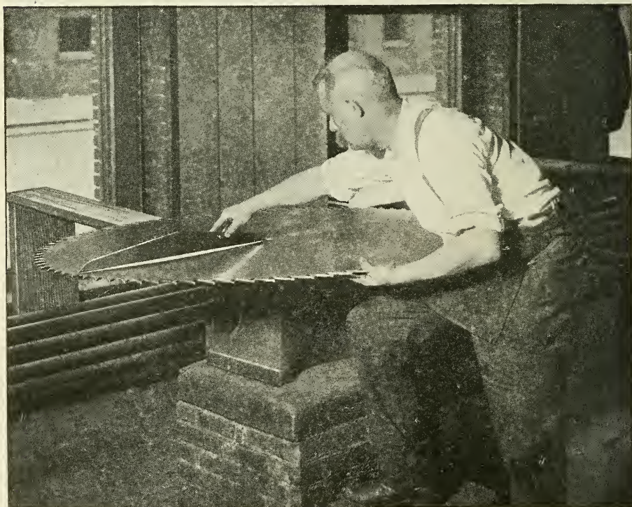
Fig. 74. Testing for tension with a short straight-edge
