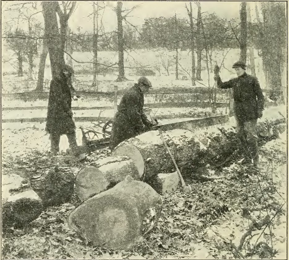
Fig. 127. A motor driven drag saw in action
