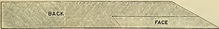
Fig. 184. This cross section of a Disston machine knife shows how the face is welded to the back
