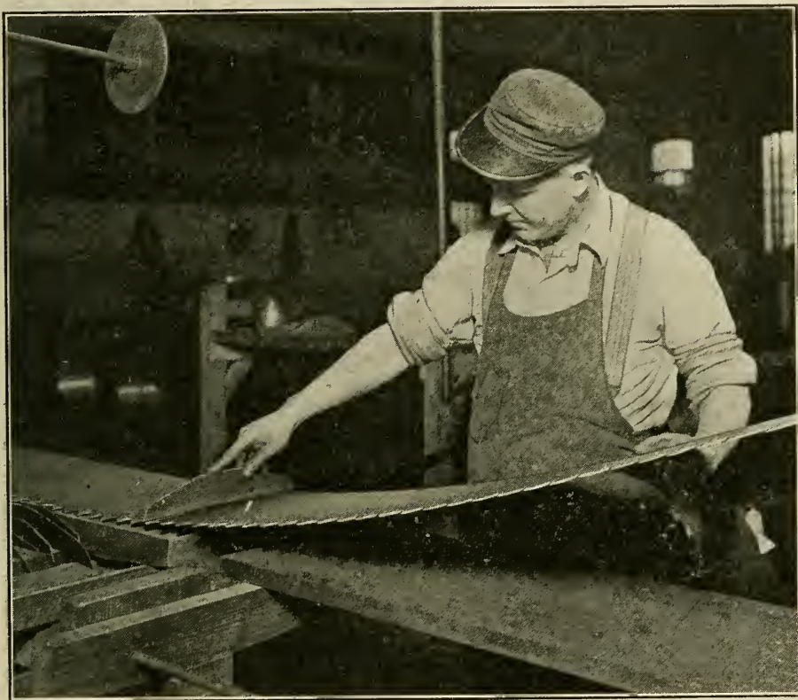
Fig. 91. "Drop" in blade fits tension gauge
