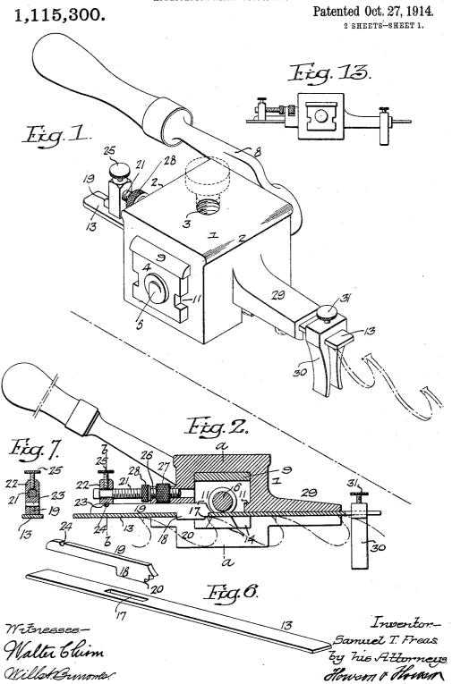
S. T. FREAS. SWAGE SHAPER FOR SAW TEETH. APPLICATION FILED OCT. 3, 1913.
